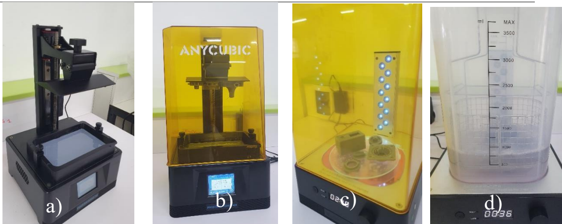
Figure 16 3-D printing Process: a) ABS-Like Resin, b) Anycubic Photon Mono 4K c) Cure Machine d) Anycubic Wash
