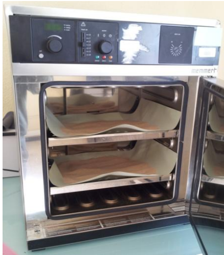
Figure 20: Etuve de séchage.
