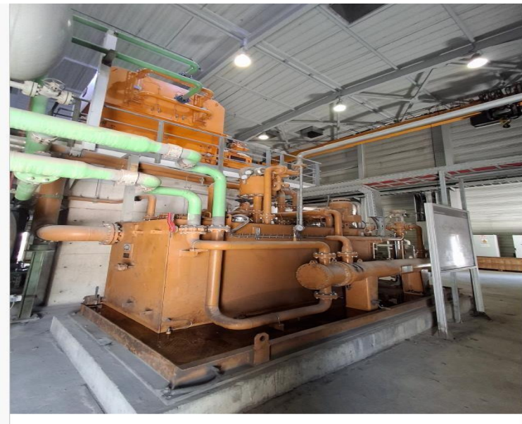
Appendix D.4: real picture of the expander - Booster in the ASU
