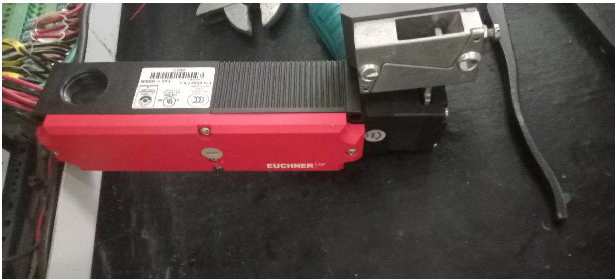
Figure 4. 8: The safety relay module and its mechanical actuator.
