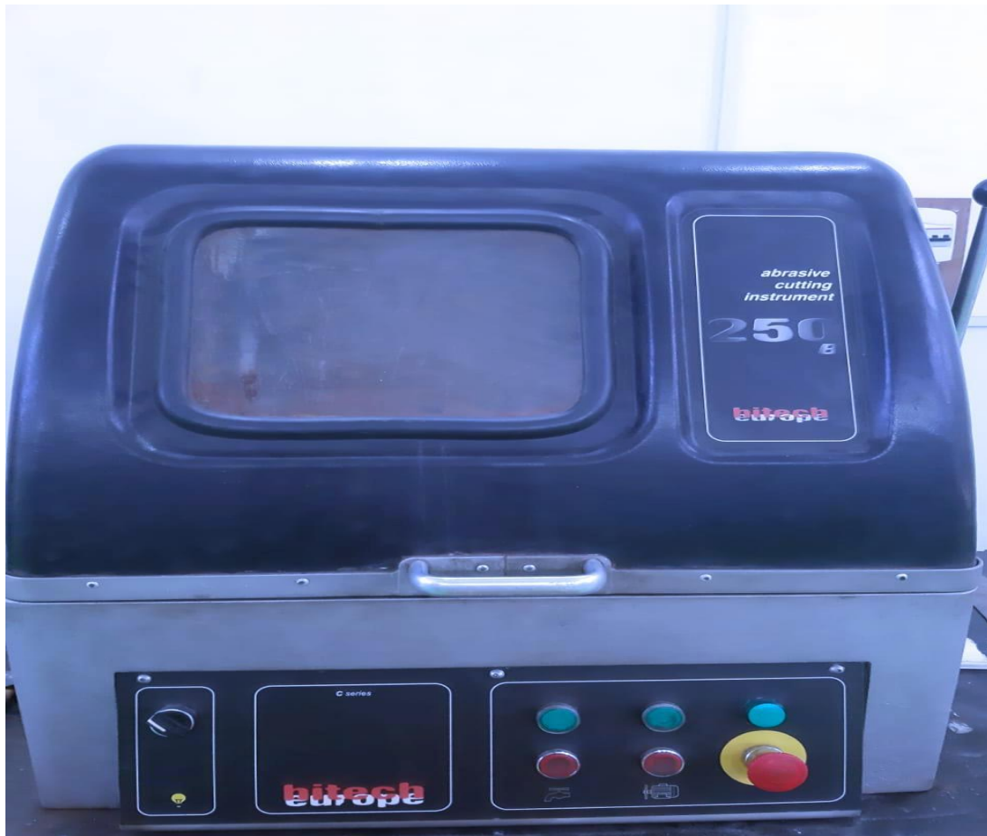
Figure 3. 3: The Hitech Europe 250 B Macro Cut-Off Saw
