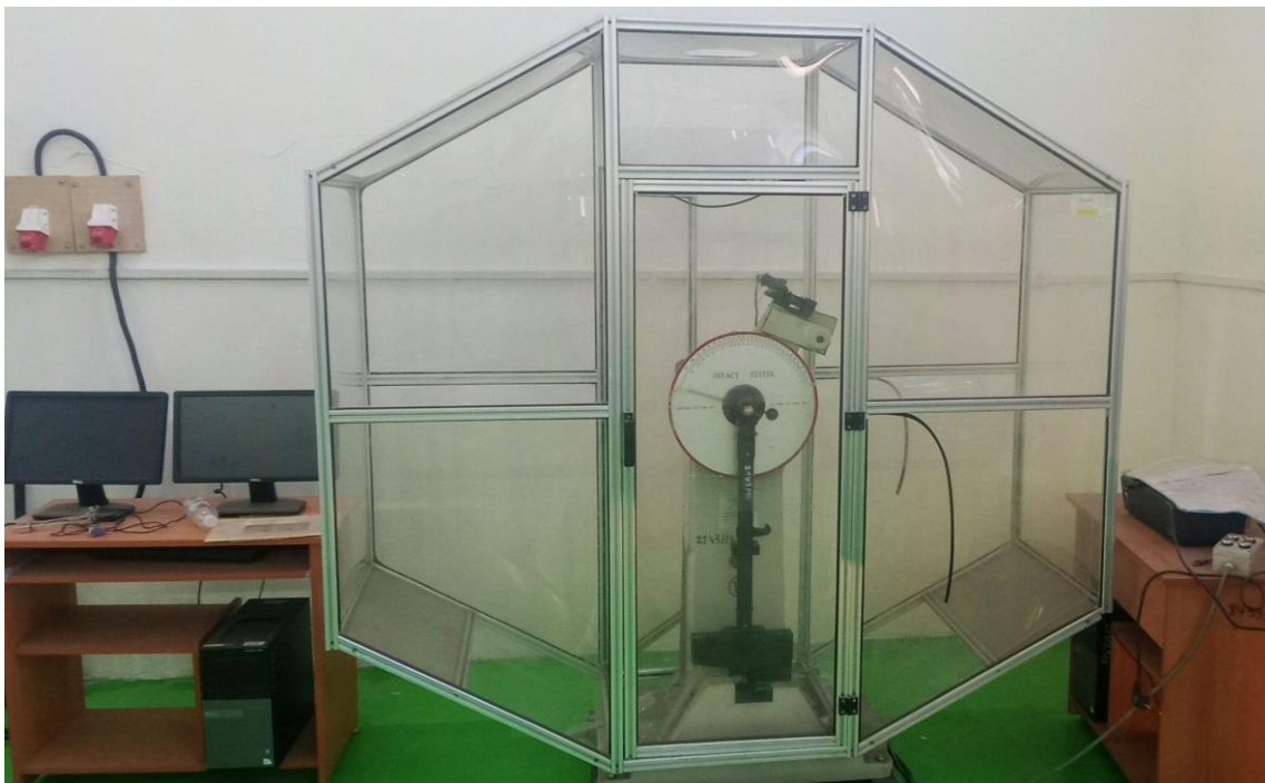
Figure 3. 4: The Impact Testing Machine (JBW-300N)
