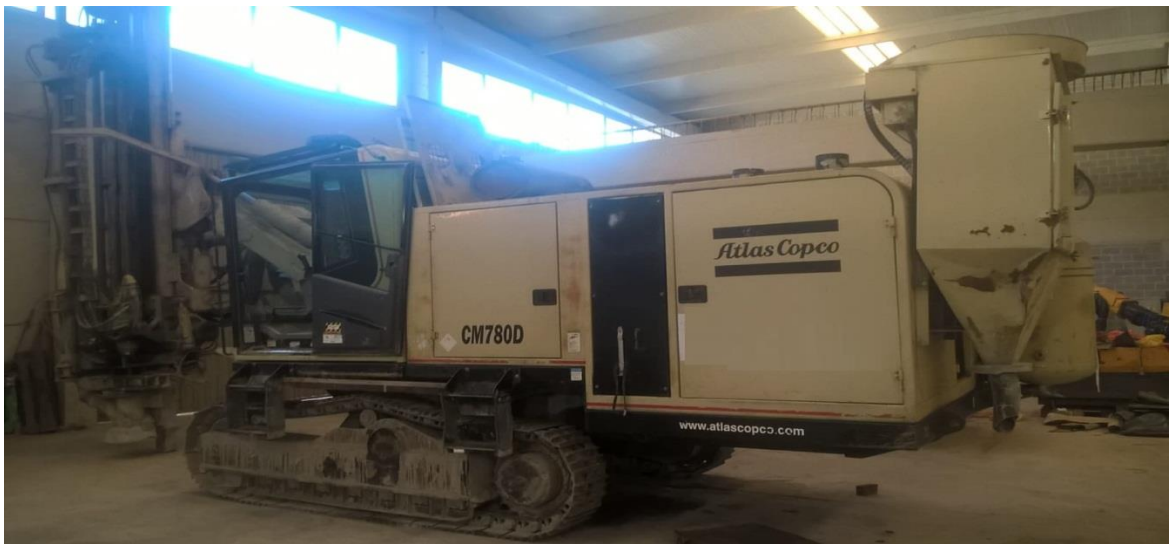
Figure III-5: sondeuse roto percutante Atlas Copco CM780D
