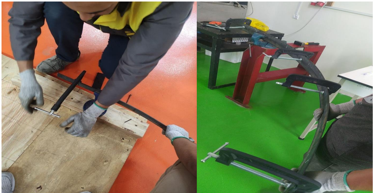
Figure 12: Manual Parabolic Shaping Adjustment of the Steel bars
