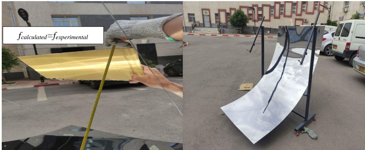
Figure 15: Precise Focal Point Adjustment Using Sunrays
