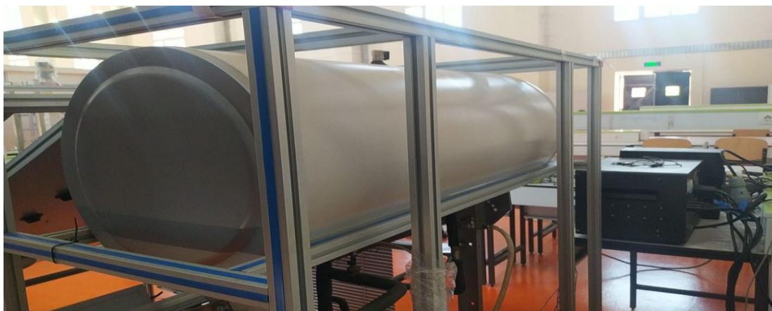
Figure 24: Thermal storage device
