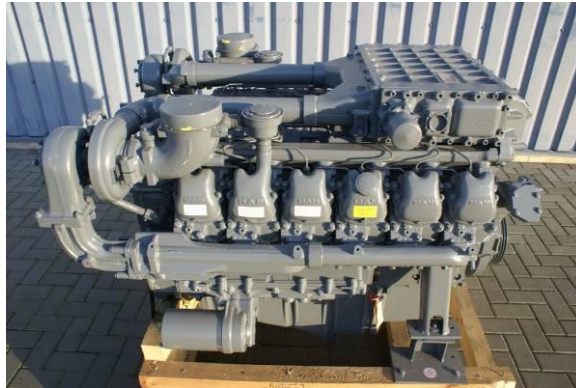
Figure II-2: Moteur diesel man d2842 LE201
