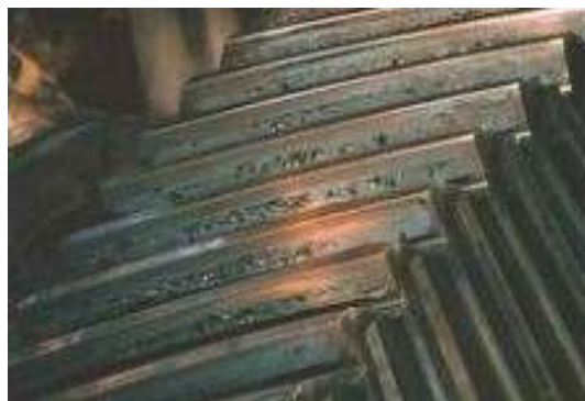
Figure 1-3 Pitting ou piqûres "Engrenages"
