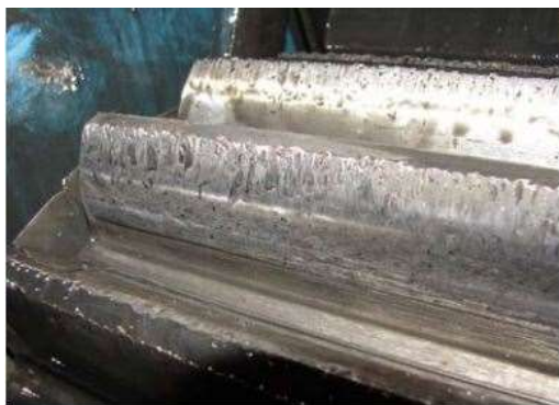
Figure 1-6 Figure Le grippage "Engrenage"
