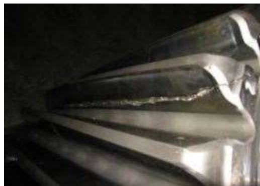
Figure 1-7 Fissuration ou cracks "Engrenages"
